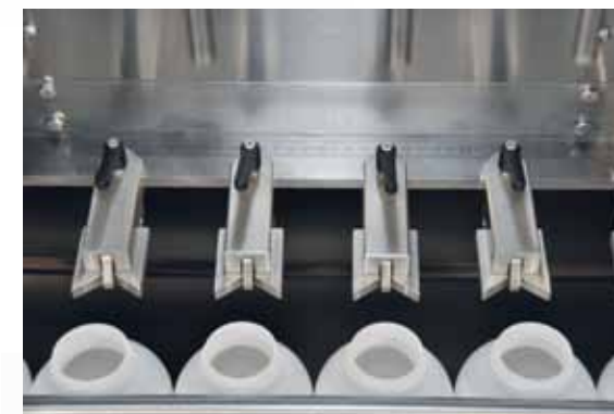
Flaschenhalsabfragung "no can, no fill"
