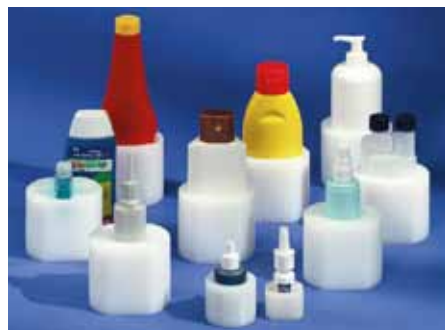
Transportbecher-System • Carrier system
